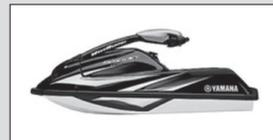
**701 Super Jet:** It is current best-selling watercraft due to its light, flat-bottom hull, powerful 701cc engine and modification-friendly nature.
