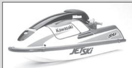
**Kawasaki 650 SX:** The next generation hull released in the mid-90's with the bigger and more potent 650cc engine than its 550 SX predecessor.
